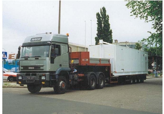
*Container power supply stations can be transported from place to place according to customer's necessity. Whole structure of the container together with such equipment like transformer and air conditioner are assembled on a support frame. It allows for safe and not difficult loading and transport.*
