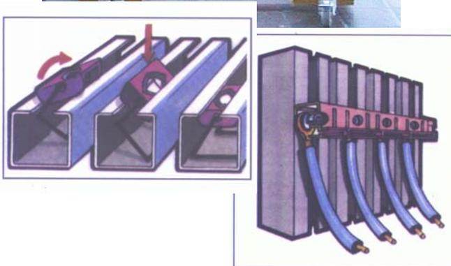
Bus-bars of load-carrying capacity from 3000 A to 7800 A are mounted in separate compartments made of standard elements of the system TABULA. It is not necessary to make drilling in order to connect horizontal and vertical bus-bars.
